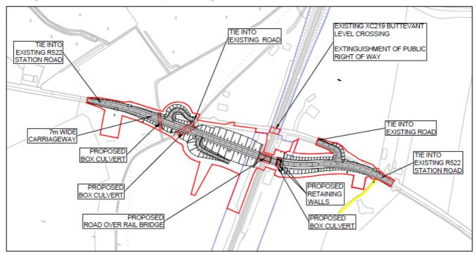
The remaining sections of the existing local road pavement to the north and south of the closed level crossing will be retained as they are required for access.
