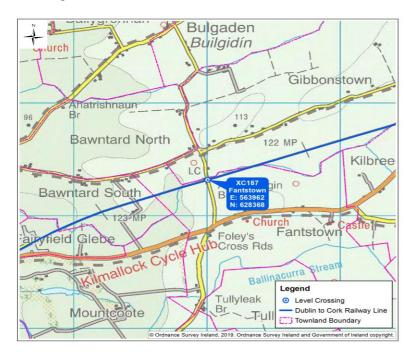
The level crossing is manned 07.30hrs-23.30hrs and the gates are normally closed to road traffic, with the gate keeper opening the gates as required. The crossings are closed to road traffic from 23.30hrs until 07.30hrs. Similar to XC201 Thomastown, the length of time that the road user is waiting depends on when they arrive at the gate and if a train has left Limerick Junction or Charleville. The road user has to wait until they pass.
