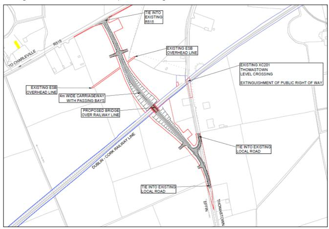
The current carriageway cross section is approximately 4m wide with 1m verges. It is proposed to provide a 4m wide carriageway with 1m verges, to tie-in with existing cross section. Verges will be widened as required for safety barrier set-back and working width. Passing bays will also be provided, as per Section 10.9 of DN-GEO-03031.
