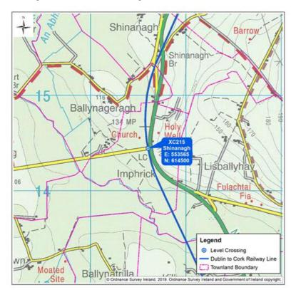
XC215 Shinangh is designated a 'CD-Type' level crossing but it has been operated as a 'CX-Type' level crossing for over 25 years and similar to XC212 Ballycoskery is manned on a 24-hour basis. Its operation as a 'CX-Type' crossing results in the gates being normally open to road traffic with the gate keeper closing the gates as required for rail traffic.
